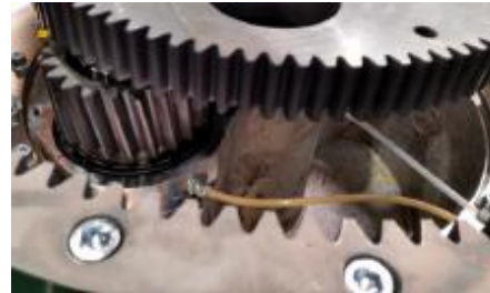
Special coating as an additional wear protection
