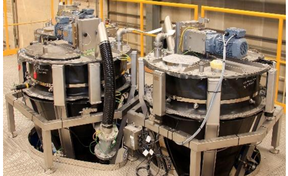
Silos with filling station, for manual and for automated refill.
