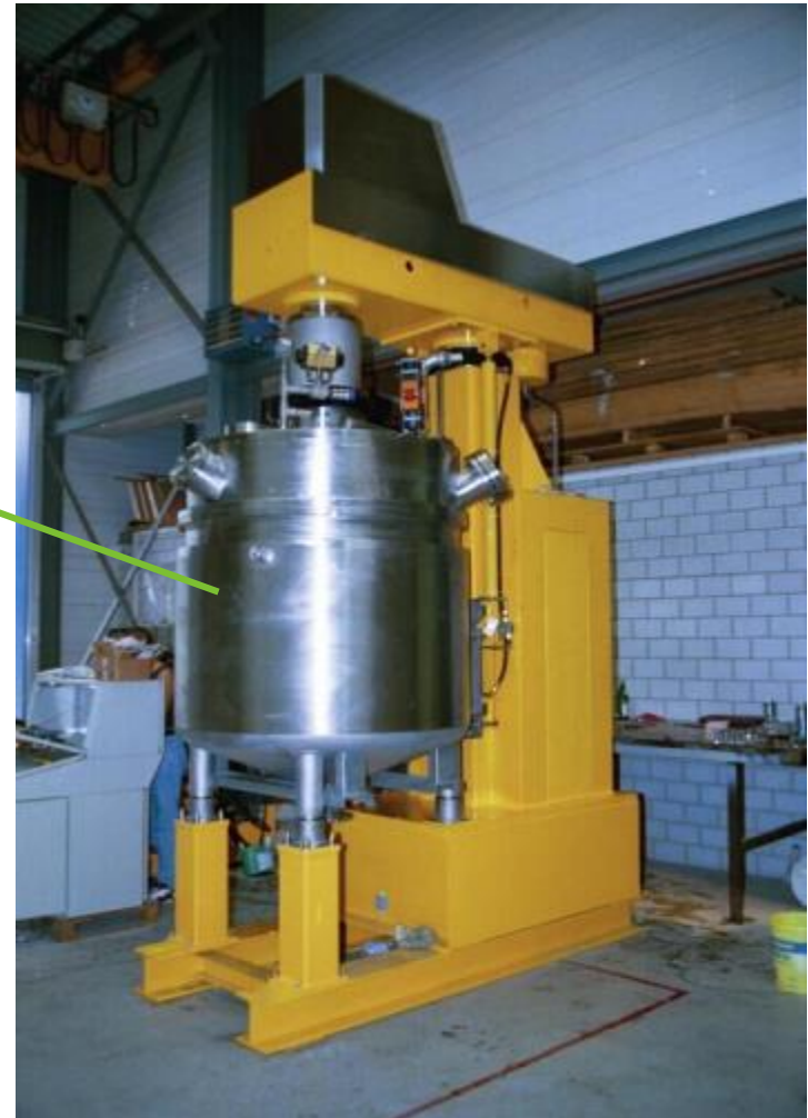
PAST mix 1000L for RTV Sealant Manufacturing, Sika AG, Germany
