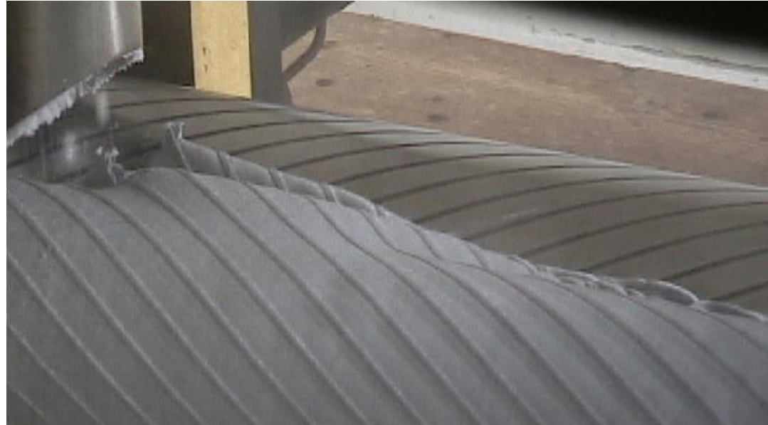
Typical PBX product felt on the rollers of an Atextruder
