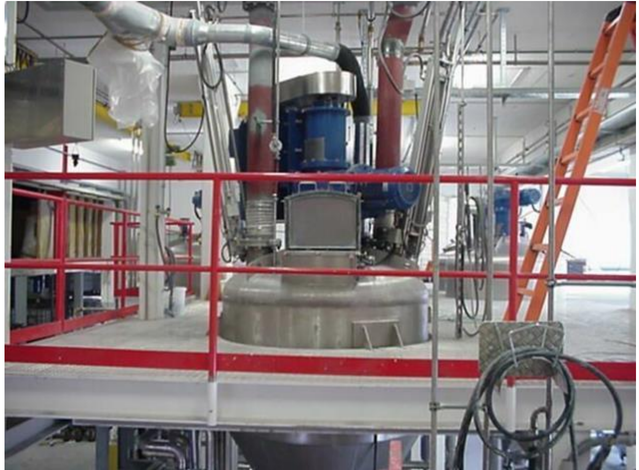
3000 L Conical Shaped Co-axial Mixer KDA for Emulsion Paints and Plasters, Greutol AG, Switzerland
