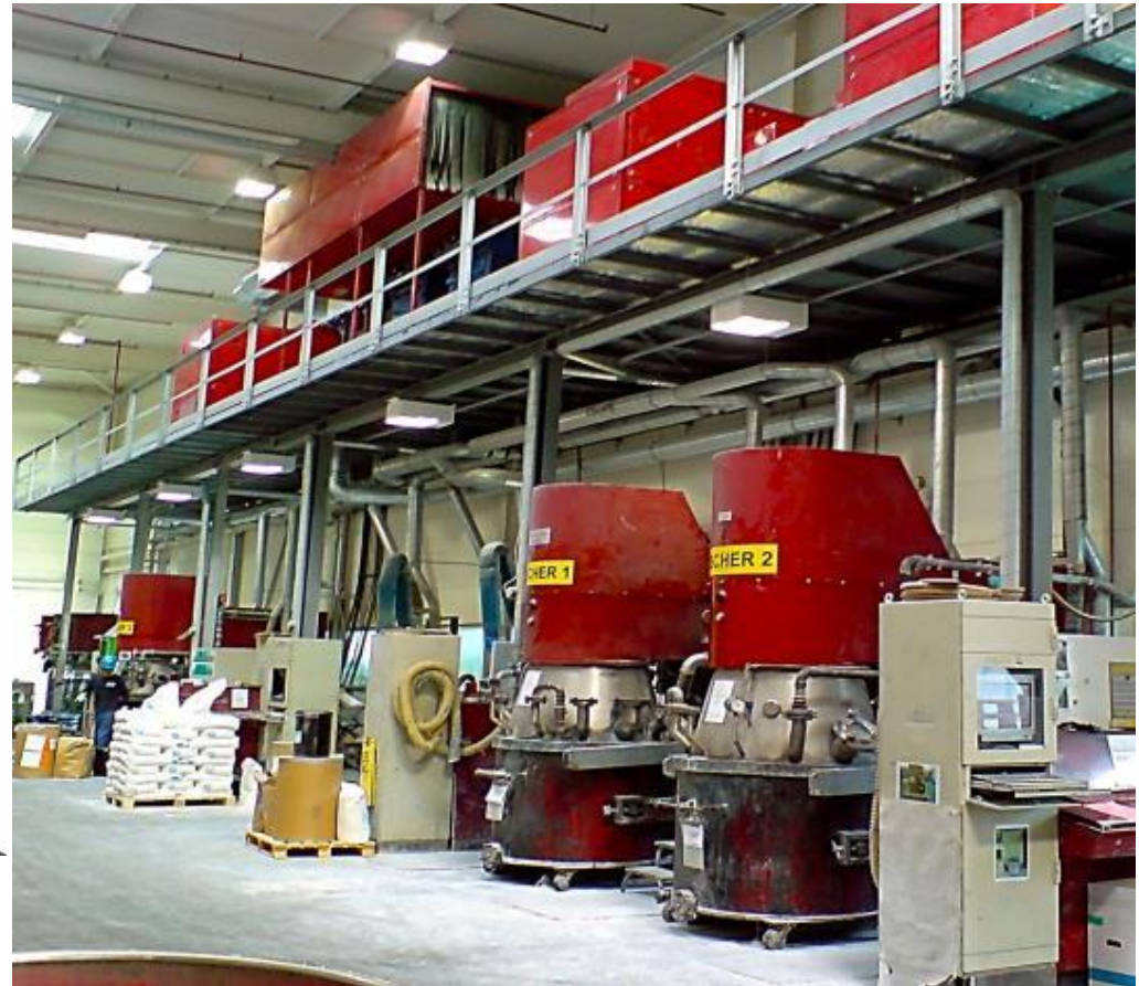
Vertical Planetary Mixer 1000 L for Automotive Adhesives, Dow, Germany
