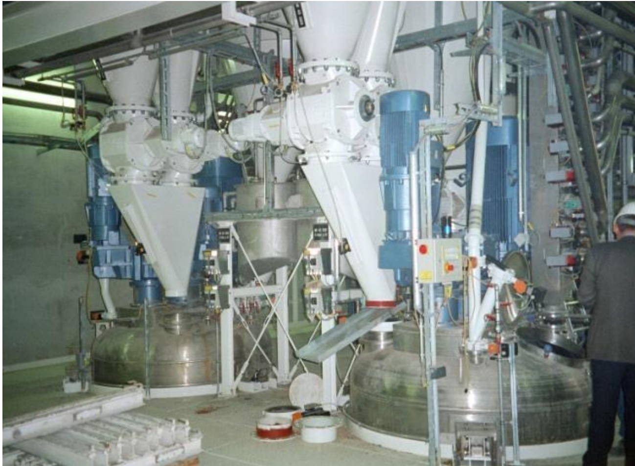
3500 L Mixing Vessel for the Production of Emulsion Plaster Production, Austria
