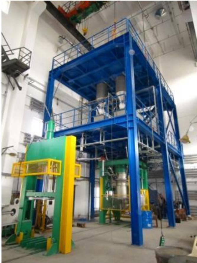
PKV 1000 Plant, high-viscous materials, incl. Bulk Material Handling and Discharge Press
