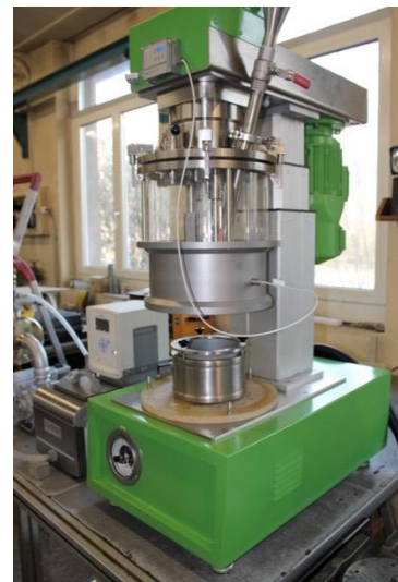
Picture 2: Open process tank Mixer 1 or 4 Liter
